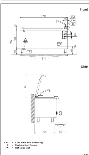
**Electric** Supply voltage: 400 V/3N ph/50/60 Hz **Total Watts:** 48.2 kW Installation: FS on concrete base;FS on feet;On base;Standing against wall;Wall mounted (with wall-kit) Type of installation:
